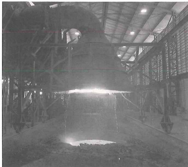
Production of ferro-niobium by thermite reaction
